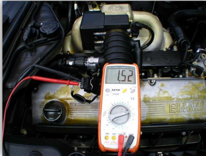
Figure 4 - Checking Air Flow voltage at idle
