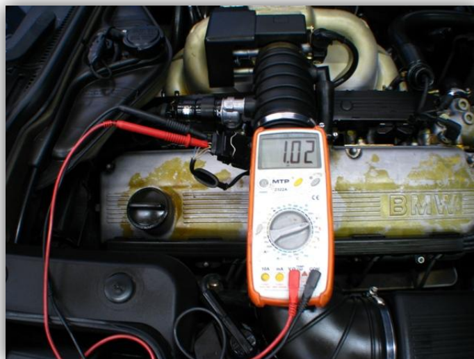
Figure 6 - Checking for Air Flow signal
