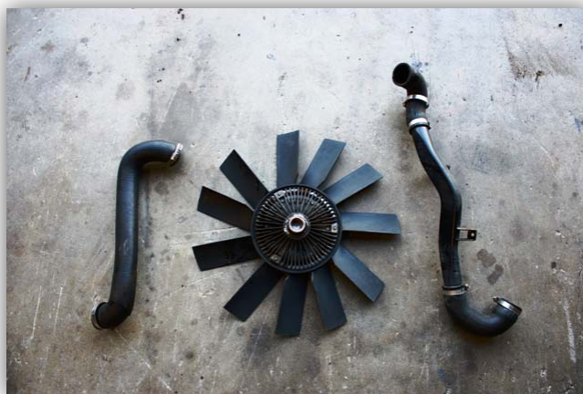
Figure 6: Items removed from E30
