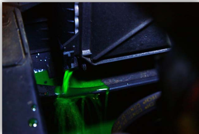
Figure 7: Coolant draining from radiator
