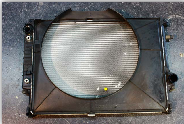
Figure 11: E34 Radiator removed
