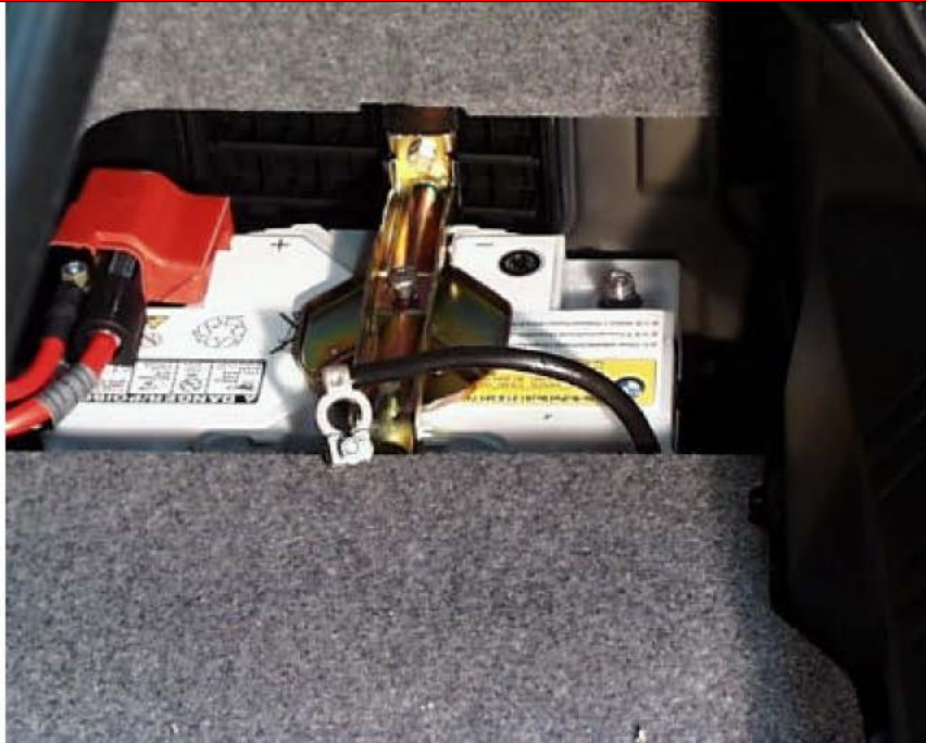
Figure 1 Disconnect the Negative terminal on the battery.
