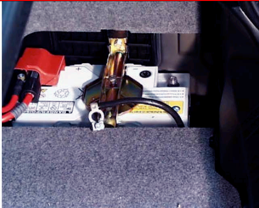
Figure 1 Disconnect the Negative terminal on the battery.
