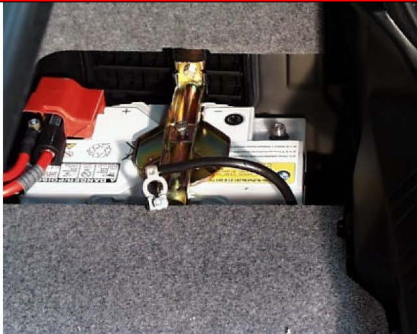
Figure 1 Disconnect the Negative terminal on the battery.
